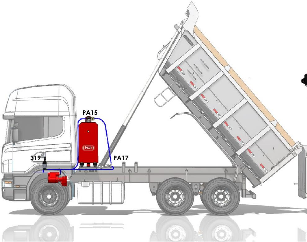
**319 - VÁLVULA NEUMÁTICA MONOCOMANDO 1/8" BSP**
